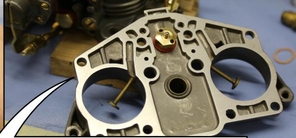
THE TOP COVER, CARBURATOR TOP AND BOTTOM ARE MADE FLAT ON A TRUE SURFACE USING SANDPAPER. TO MAKE THE SURFACES NICE AND SMOOTH I WENT FROM 300 GRIT UP TO 1000 GRIT. THIS WILL PREVENT ANY LEAKAGE OF AIR OR FUEL.
