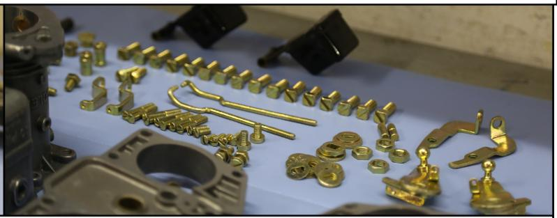
ALL JETS ARE MEASURED AND CLEANED. THE HARDWARE IS REPLACED IN THE ORIGINAL YELLOW ZINC. THE ADJUSTMENT BLOCKS IN BETWEEN THE THROTTLE SHAFTS ARE REPLACED. THESE ARE OFTEN WORN AND BENT. SHIMS ARE USED AT THE ENDS OF THE SHAFTS IN ORDER TO GET THE BUTTERFLY TO ROTATE EXACTLY IN THE MIDDLE OF THE BORE.
