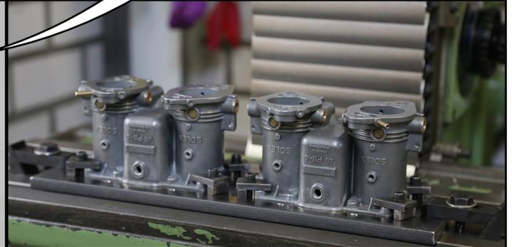
THE THROTTLE BORES ARE MILLED TO OVERSIZE IN ORDER TO MAKE THE NEW BUSHINGS FIT THE RADIUS OF THE BORE. IN THIS PROCESS THE GROOVE THAT THE PREVIOUS BUTTERFLY CAUSED WILL ALSO BE REMOVED. I WAS ABLE TO MAKE THE BORES CLEAN AND ROUND BY MILLING TO AN OVERSIZE OF 40,5MM. SHOULD THEY NEED AN OVERHAUL IN THE FAR FUTURE THEY CAN BE OVERSIZED TO 41MM.
