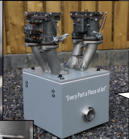
THE LAST ADJUSTMENT STEP IS TO MAKE SURE THAT THE AIR FLOW THROUGH ALL FOUR BORES OF THE CARB IS THE SAME. A VACUUM BOX IS USED WITH A 1500 WATT MIELE VACUUM CLEANER TO PROVIDE THE VACUUM NEEDED.
