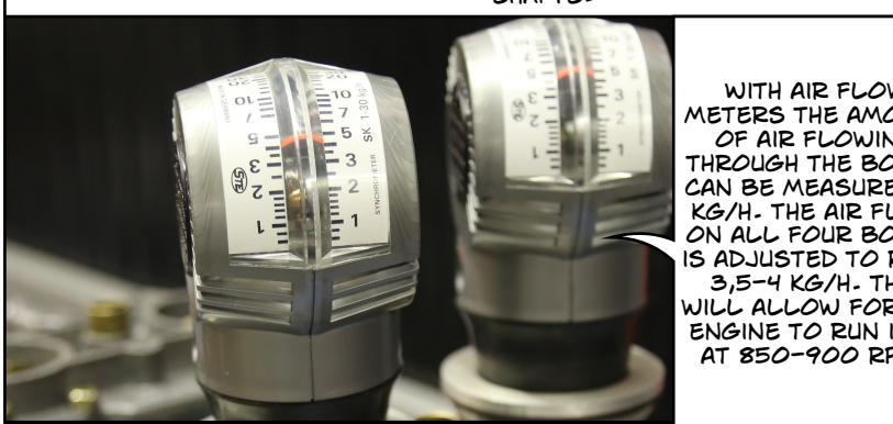
WITH AIR FLOW METERS THE AMOUNT OF AIR FLOWING THROUGH THE BORES CAN BE MEASURED IN KG/H. THE AIR FLOW ON ALL FOUR BORES IS ADJUSTED TO READ 3,5-4 KG/H. THIS WILL ALLOW FOR THE ENGINE TO RUN IDLE AT 850-900 RPM.
